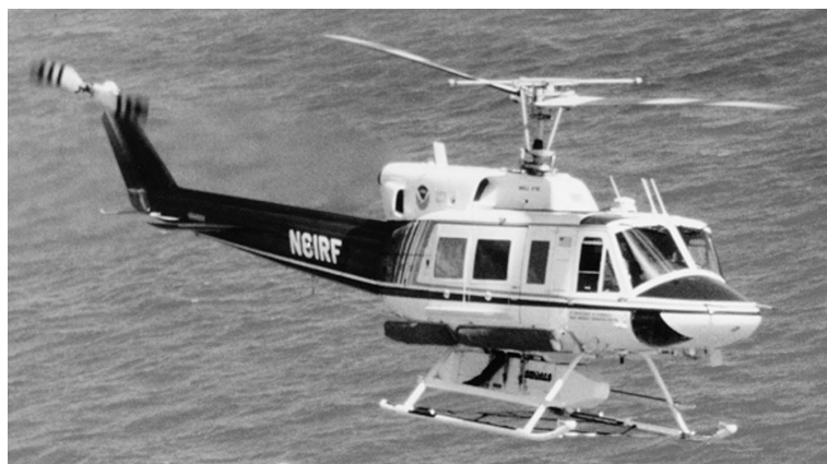
Fig. 2. The SHOALS system mounted on underside of a Bell 212 helicopter.
