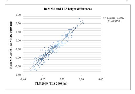
Figure 6. Correlation between TLS- and BoMMS-derived elevation changes.
