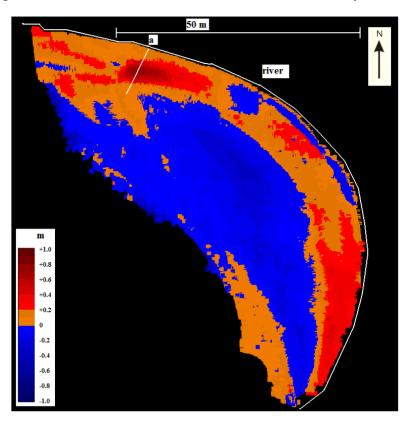
Figure 7. Deposition and erosion areas on Point Bar 2 between the years 2009 and 2008.
