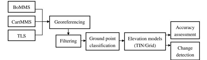
Figure 3. The processing chain for point cloud data.
