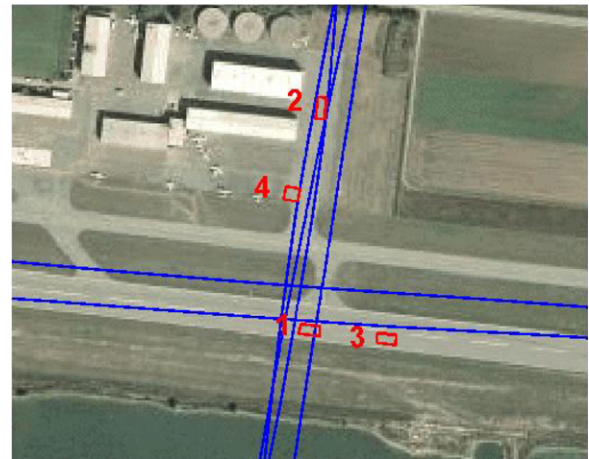
Fig. 13. Calibration airfield with tracks (blue) and calibration areas (red). (For interpretation of the references to colour in this figure legend, the reader is referred to the web version of this article.)
