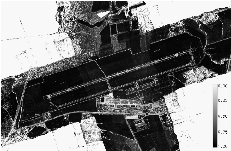
Fig. 2. r -square of the local LSA for an empirical model. Low r -square values in the image corners are mainly due to the small number of strips covering these areas, hence resulting in a small number of points and few distinguishable ranges per cell (3 m cell size).
